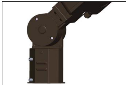
Slipfitter Mount An optional cast aluminum mast arm adapter secures fixture head to nominal 2"(2-3/8" O.D. pipe size) horizontal steel tenon arm.
